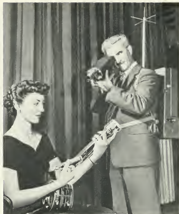
Development of Vidicon tube (in girl's right hand) made possible the back-pack TV transmitter shown at right.
